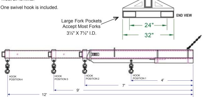
CAUTION: BE AWARE THAT FORKLIFT RATED CAPACITIES <u>DIMINISH RAPIDLY</u> WHEN THE LOAD CENTER IS MOVED OUT. WHEN USING THE JIB, MAKE SURE YOUR FORKLIFT HAS ADEQUATE CAPACITY TO HANDLE THE DESIRED EXTENDED LOAD. SEE BOTH THE HEAVY DUTY JIB AND YOUR FORKLIFT OPERATOR'S MANUALS FOR MORE INFORMATION. LOAD CAPACITIES SHOWN HERE ARE FOR THE JIB ITSELF AND DO NOT IN ANY WAY REFLECT THE LIFT CAPACITY OF THE FORKLIFT.
